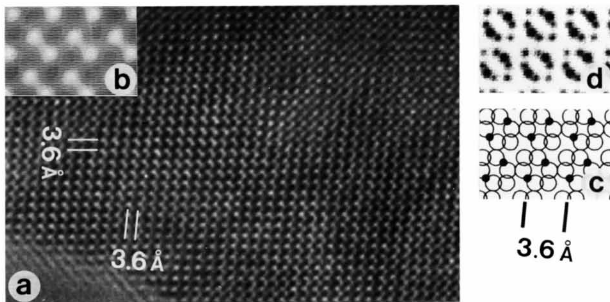
Fig. 2. [2\bar{2}1] lattice image ( a ) with the corresponding simulated image ( b ) at the crystal thickness z = 50 \text{ \AA} and the defocus value \Delta f = 550 \text{ \AA} . ( c ) Projected structure: dots and circles designate columns of vanadium and oxygen atoms, respectively. ( d ) Projected potential distribution: the dark part corresponds to a higher-potential area. The nearest-neighbour columns (separated by 2.1 \text{ \AA} ) of vanadium atoms are not resolved and are situated in the dark area in the image ( a ).
