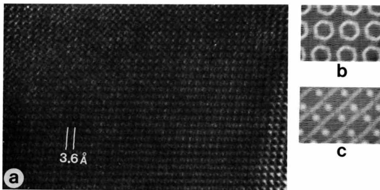
Fig. 5. (a) [2\bar{2}1] lattice image where the crystal thickness increases from lower right corner to upper left. In the intermediate region, an array of small white circles having a diameter of ca 1.7 Å is visible. (b) A simulation at z = 100 Å and \Delta f = 1350 Å in the perfectly coherent case. (c) A simulation ( z , \Delta f the same as above) with the finite partial coherence allowed for by the intensity-sum method (see text) taking u_s = 0.030 Å -1 and \sigma = 50 Å.
